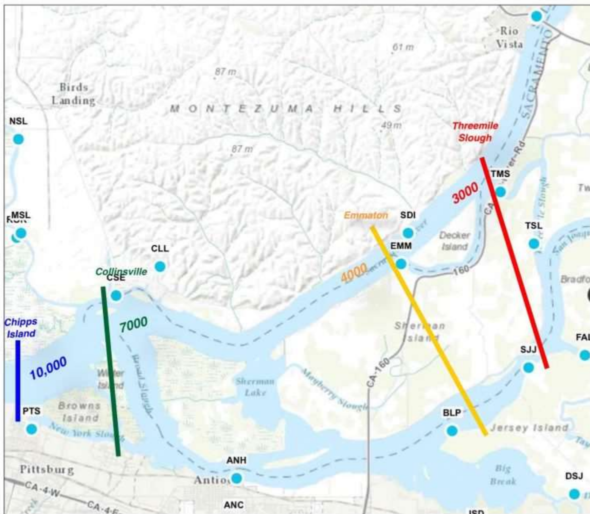
Figure 1. Location of X2 (2 parts per thousand salinity) in the Delta at various Delta outflows.
